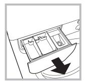
Remove the dispenser by raising it and pulling it out (*see figure*). Wash it under running water; this operation should be
